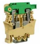
The terminal block is fitted with a lever which enables insertion of a  $\emptyset$  6.3 x 32 mm - 500 V fuse and a neon light with resistance incorporated (our type LSN  $\emptyset$  6 x 26 mm - 380 V max).
