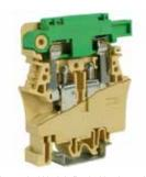
The terminal block is fitted with a lever which enables insertion of a  $\emptyset$  6.3 x 32 mm - 500 V fuse and a non-polarised LED microcircuit. The LED comes on to warn that the fuse is broken. The terminal block can be supplied already with the CIL circuit mounted for inserting a non-polarised LED circuit.
