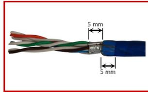
Fix the braid by use of insulating tape. 5 mm of braid have to remain uncovered to ensure the contact to the jack. Remove foil around pairs. 5mm of foil need to remain.
