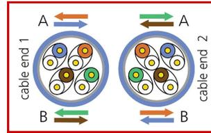
Cross the pairs acc. to TIA/EIA 568 A or TIA/EIA 568 B (see color-code on contact-block).
