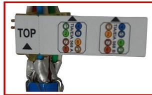
Insert the shortened pairs. Slip contactblock up to the foil.
