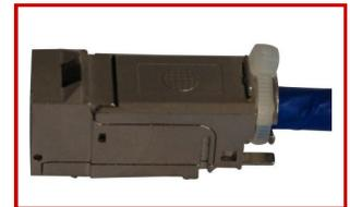
Fix jack to the cable by use of the included cable-tie.
