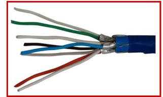
Open the twist of the pairs up to the foil.
