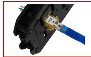
Insert contactblock with cable into the plier HSLTOOL02.
